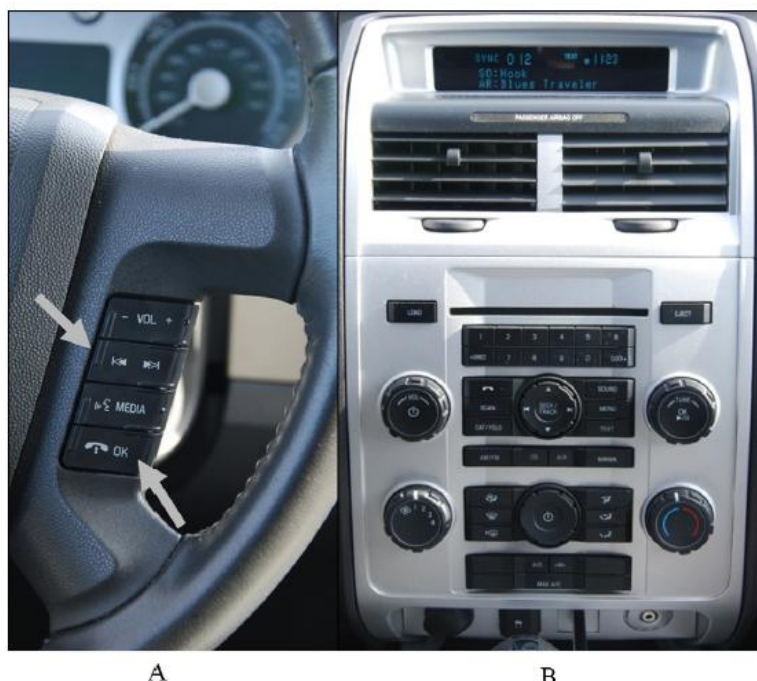
Fig. 1. Layout of vehicle system interface. (A) depicts the control buttons on the steering wheel; the arrow buttons select from options presented on a screen located at the top of the center stack (B), while the "OK" button confirms selections.
