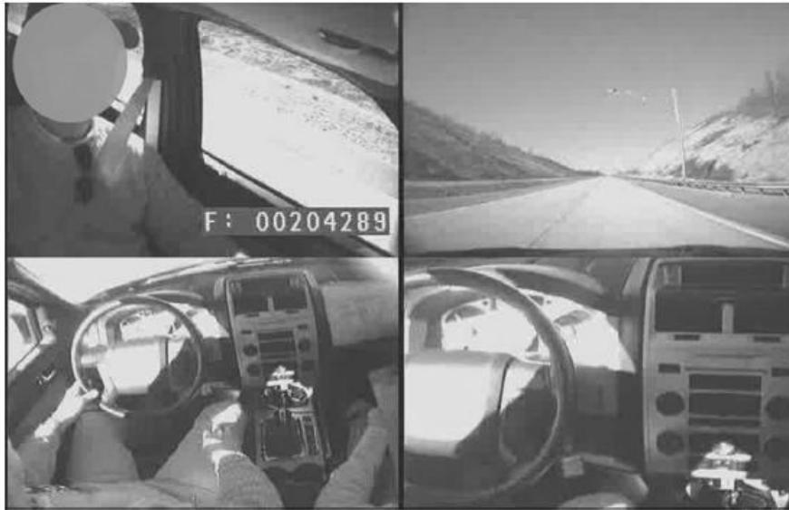
Fig. 2. Camera views of driver (face is not blurred in actual video), forward roadway, and wide- and close-views of driver's hands and center stack.
