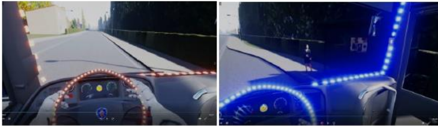
Automation at docking at bus stop. Hand/Take over in amber, automation mode in blue
