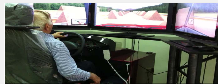
FIGURE 3. Test condition TC3, as barriers narrow the road to a single lane.
