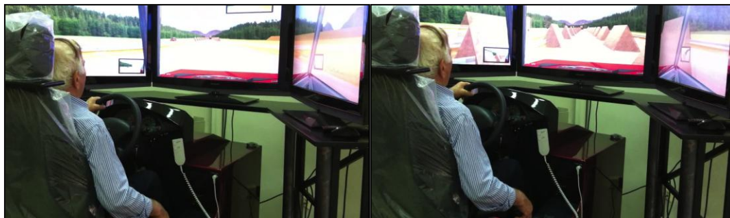
Fig. 2. Test condition TC2 (a:left) with a road works section visible in the distance; (b:right) as barriers narrow the road to a single lane.
