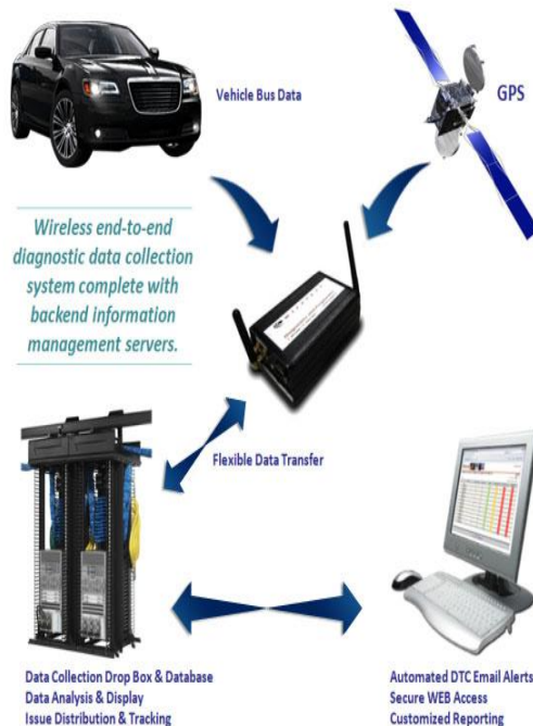
Fig.1. Continuous data transmission from the vehicle bus via the OBD device and the GSM
