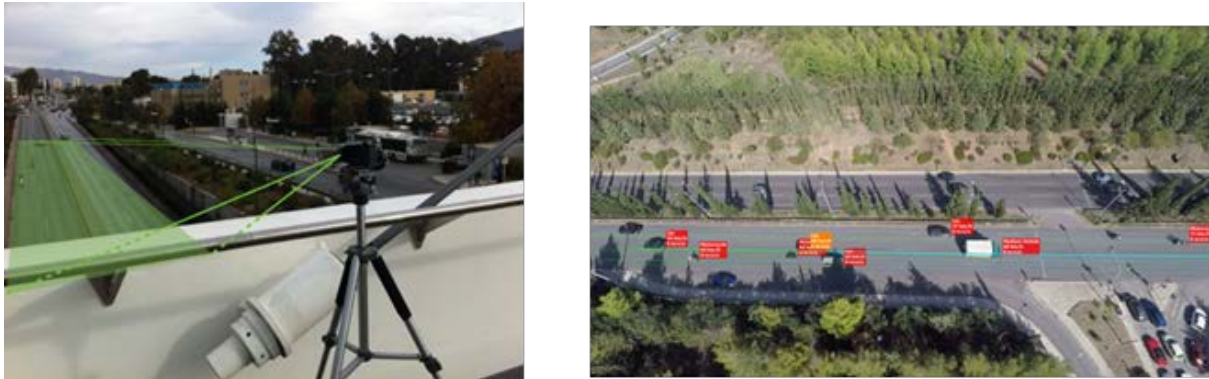
Figure 1 – Recording limited length using one fixed VS recording using a UAS over an extended area
