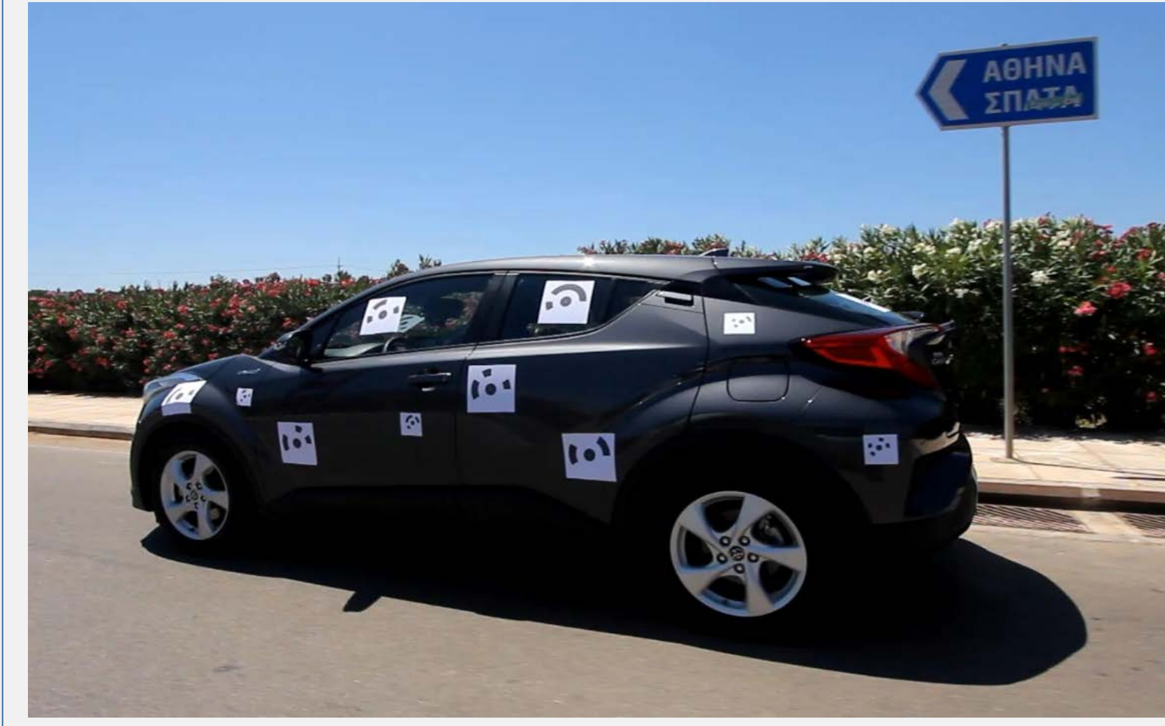
Figure 2 Coded targets mounted on the passed vehicle surface
