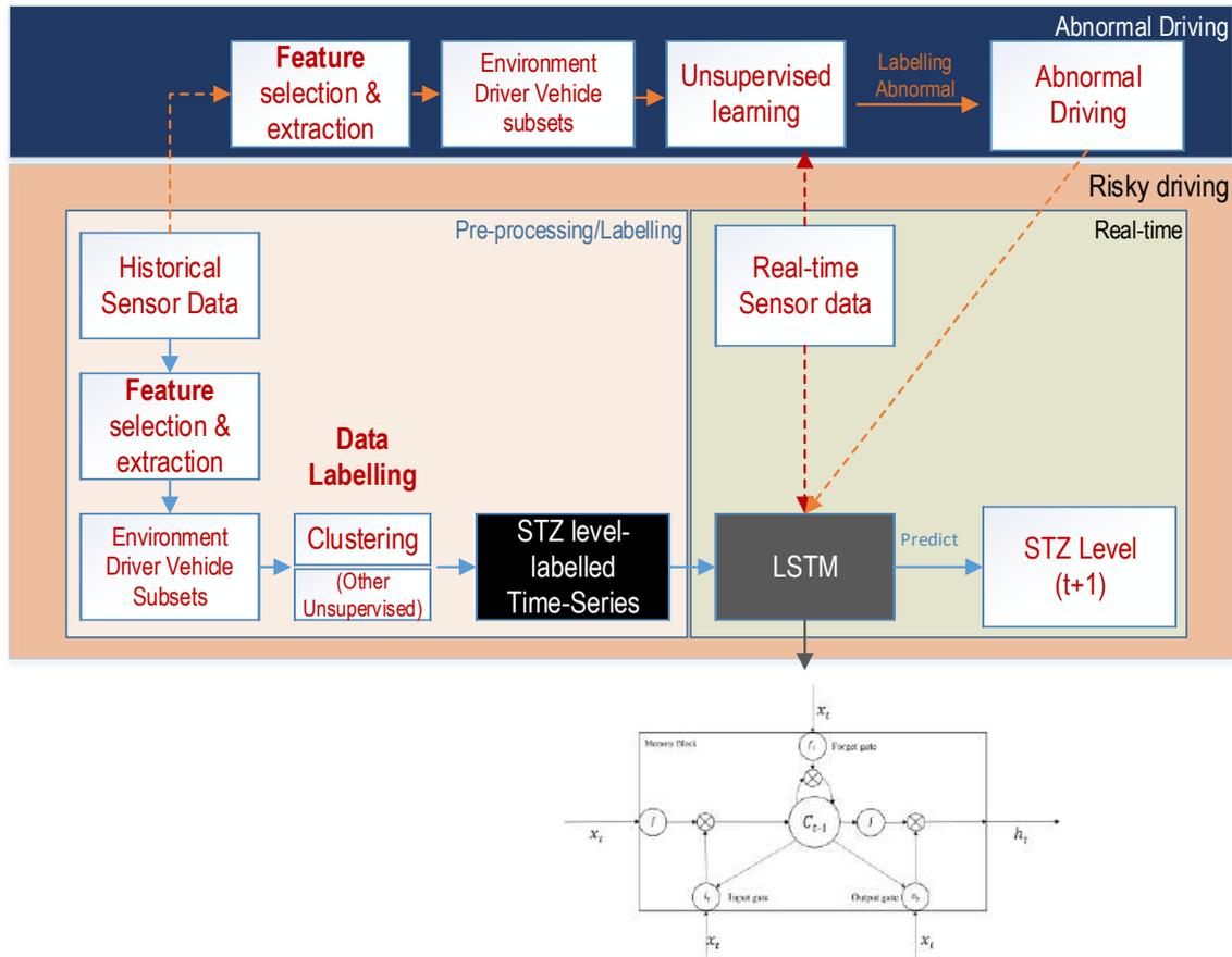
**Figure 4: STZ modelling using LSTMs**
