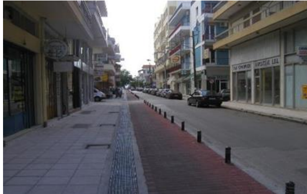
Figure 3: Segregated pedestrian – cycling traffic.
