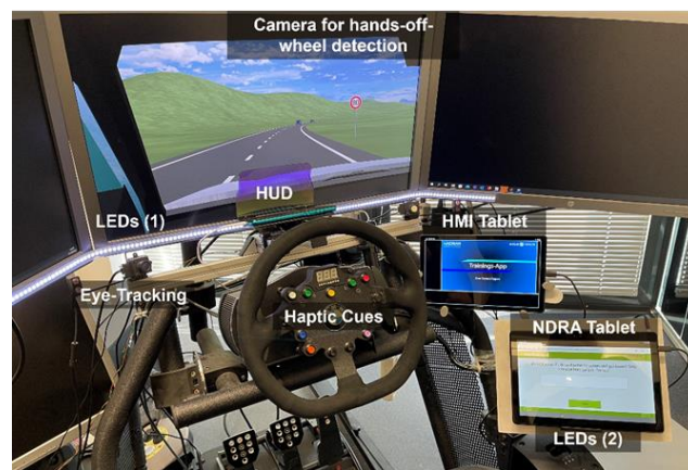
Figure 2: Components of the integrated fluid HMI of the VIF holistic study
