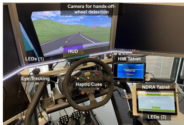
Fig. 1. Components of the integrated fluid HMI of the “Virtual Vehicle” holistic study.
