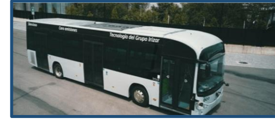
Autonomous electric bus – Irizar SAE L4
