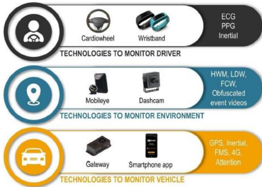
5 6 7 Figure 2 Technologies to monitor driver, environment and vehicle state 8
