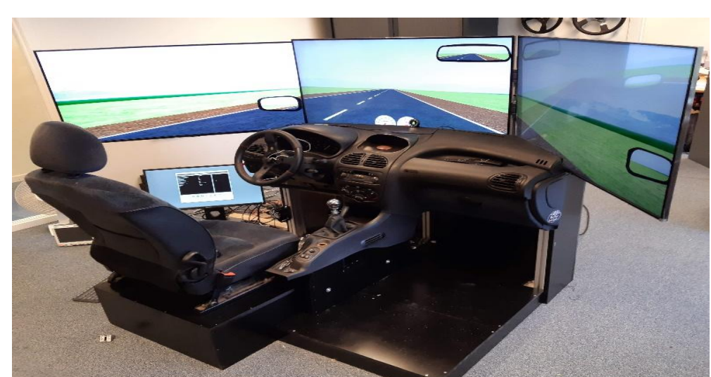
Figure 3: Car simulator developed by DriveSimSolutions, using OEM Peugeot 206 parts
