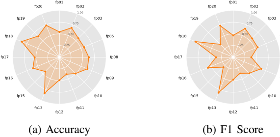
Fig. 2: Per-subject CNN-LSTM performance under leave-one-subject-out (LOSO) cross-validation. Radar plots depict (a) accuracy, and (b) F1 score for each test subject, illustrating the substantial inter-subject variability.
