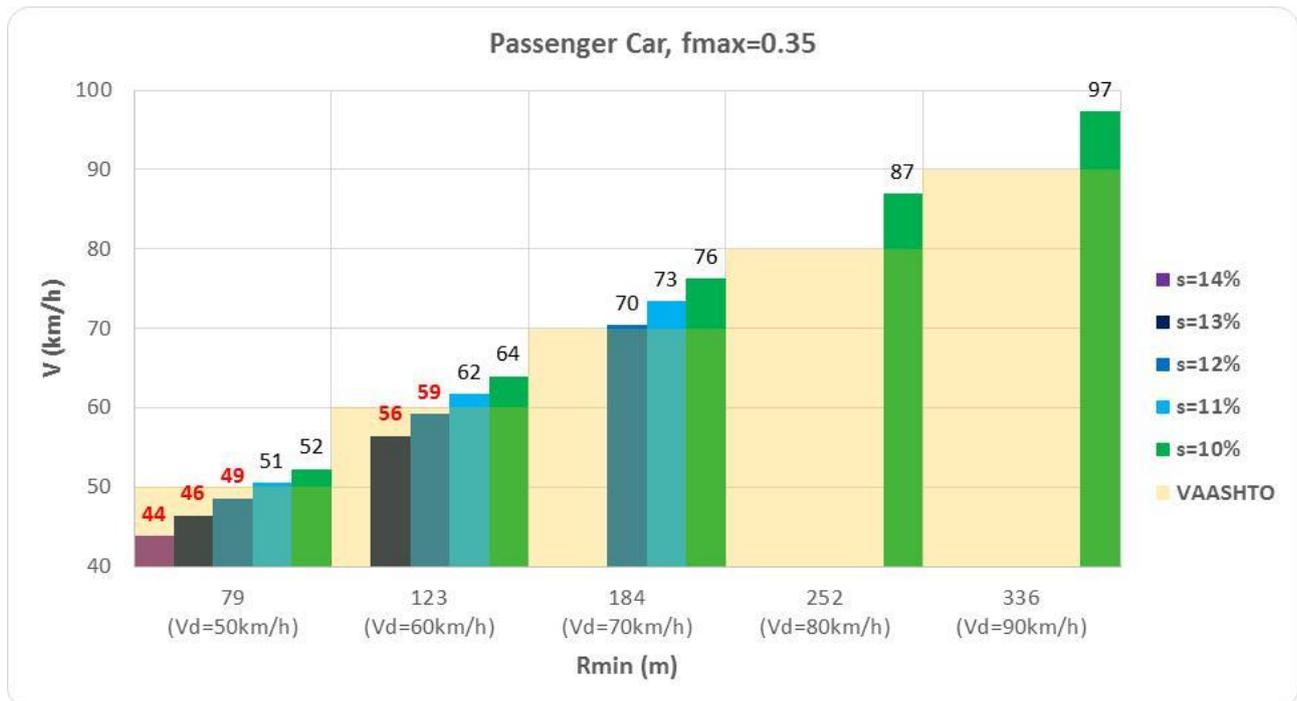
**FIGURE 1**  $V_{safe}$  Variation for Passenger Car on Poor Friction Pavement ( $f_{max}=0.35$ ).
