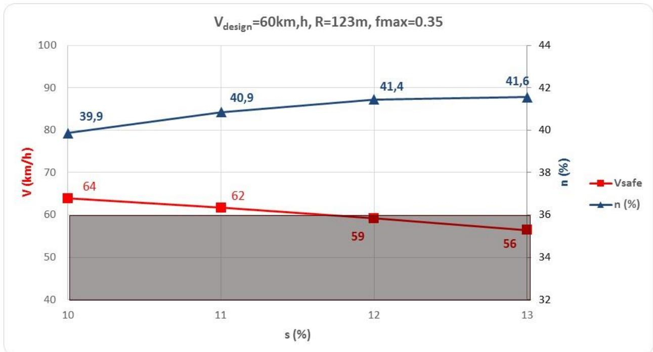
**FIGURE 2**  $V_{safe}$  Variation vs Grade Values for  $V_d=60\text{km/h}$ ,  $R=123\text{m}$ , ( $f_{max}=0.35$ ).
