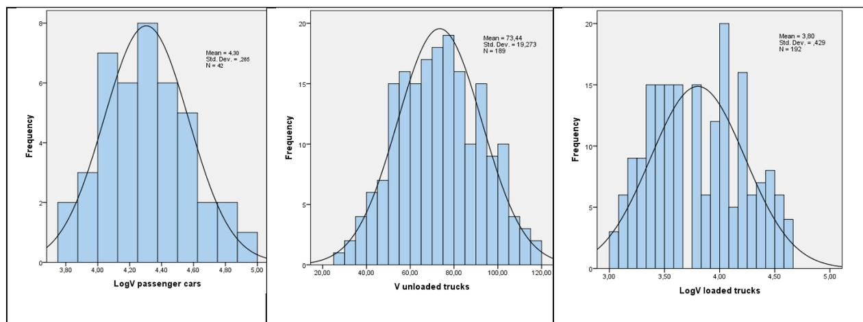
**FIGURE 4. Histograms of vehicle speed frequencies vs. normal distribution curves - Passenger car (left panel), unloaded truck (middle panel), and loaded truck (right panel)**
