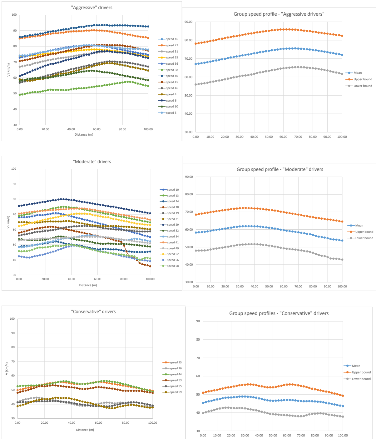
Figure 3: Speed profiles for “aggressive” (top panel), “moderate” (middle panel) and “conservative” (bottom panel) drivers - Individual profiles (left panel), group profiles (right panel)
