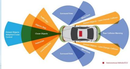
Long Range RADARs 🛛 📕 LIDAR, SRR 🛛 🔳 Camera – Stereo, Monocular 🖉 Ultrasonic Sensc
