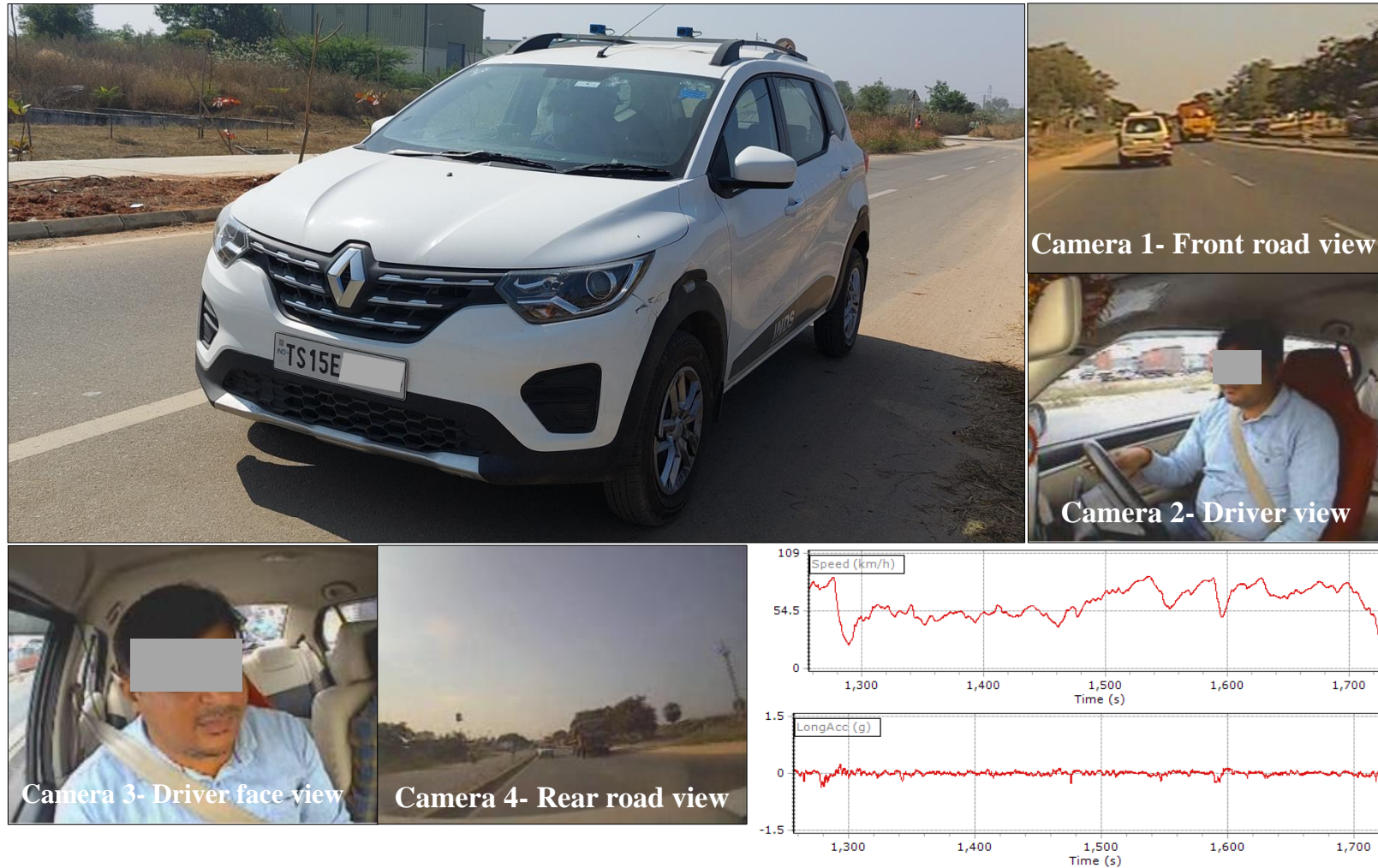
Figure 3. Study vehicle; Snapshots of collected video data; Recorded speed and acceleration profiles
