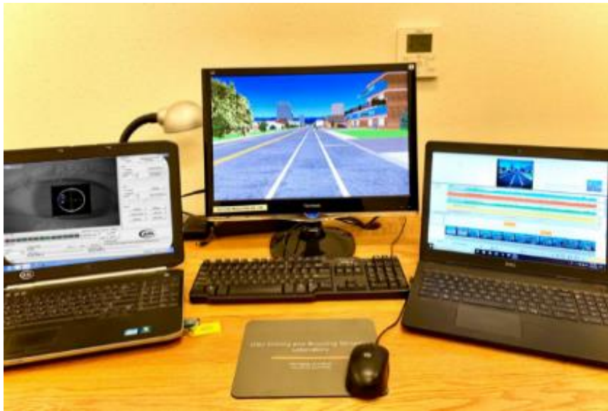
Right: Eye tracker laptop; Middle: Bicycle simulator workstation; Left: iMotions laptop
