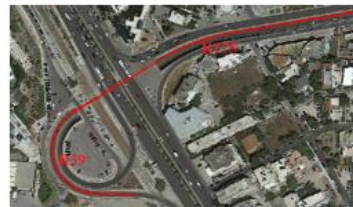
Alimou Interchange, 175 and 39 meters radii horizontal curves (trumpet)
