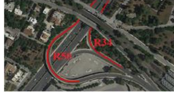
Kimis Interchange, 34 and 50 meters radii horizontal curves (trumpet)
