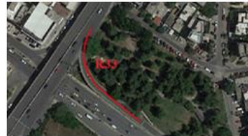
Kapodistriou Interchange, 33 meters radius horizontal curve (diamond part)
