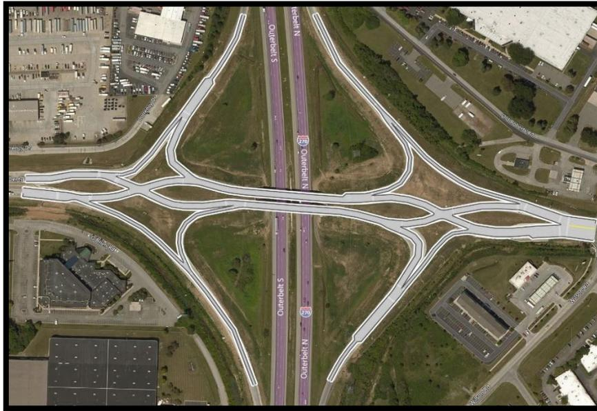
**Figure 4: The proposed diverging diamond interchange design in Vistro.**
