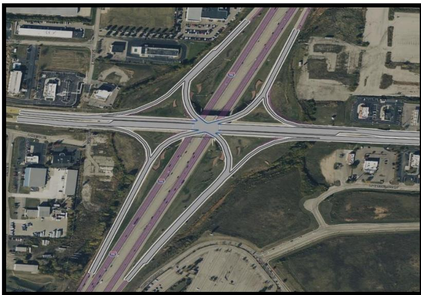
**Figure 3: The proposed single point urban interchange design in Vistro.**
