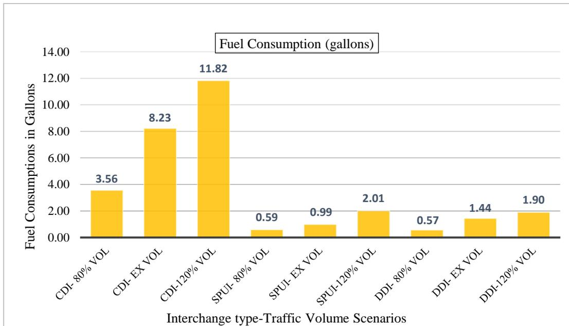
**Figure 10: Total fuel consumption in gallons for each interchange design type and traffic scenario.**
