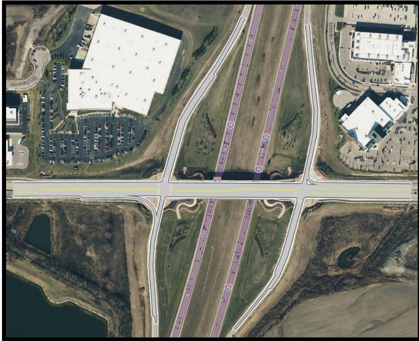
**Figure 2: The existing conventional diamond interchange design in Vistro.**
