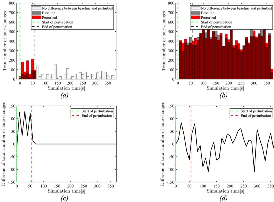
Figure 7 (a): Total number of lane changes over the whole simulation space versus time: “frozen” mode; (b): Total number of lane changes over the whole simulation space versus time: “warm” mode; (c): Difference of total number of lane changes over the whole simulation space versus time: “frozen” mode; (d): Difference of total number of lane changes over the whole simulation space versus time: “warm” mode.
