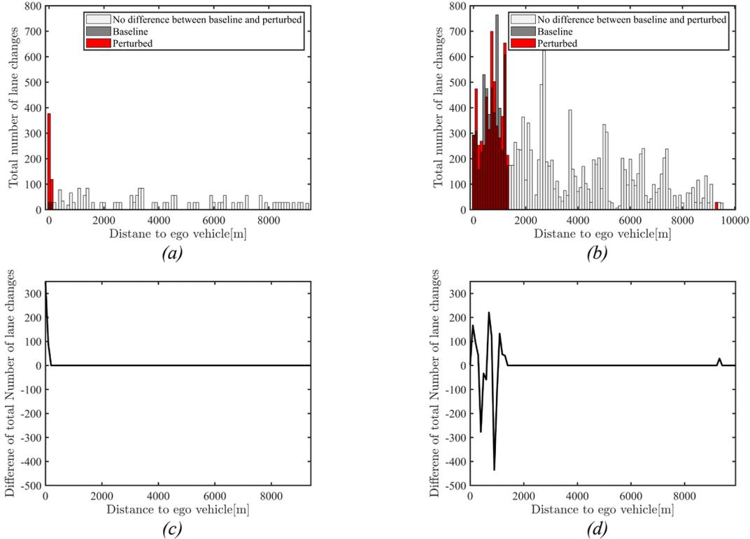
Figure 8 (a): Total number of lane changes over the whole simulation time versus distance to ego vehicle: “frozen” mode; (b) Total number of lane changes over the whole simulation time versus distance to ego vehicle: “warm” mode; (c) Difference of total number of lane changes over the whole simulation time versus distance to ego vehicle: “frozen” mode; (d) Difference of total number of lane changes over the whole simulation time versus distance to ego vehicle: “warm” mode.
