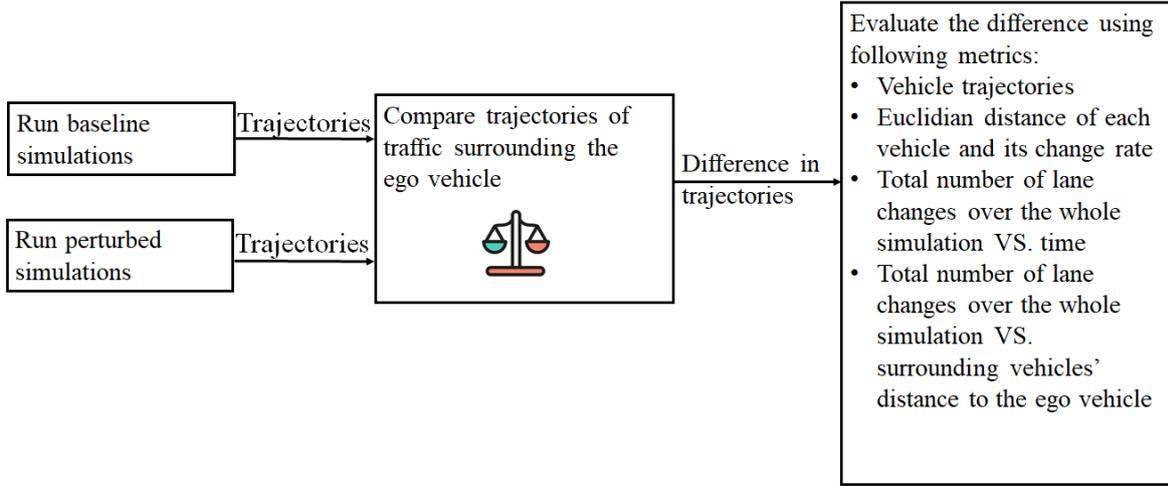
Figure 3 Analysis flow of ROI of ego vehicle on surrounding traffic.
