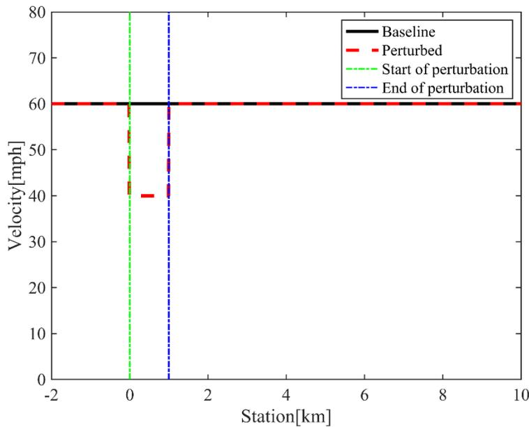
Figure 2 Velocity settings of ego vehicle in baseline and perturbed simulations.
