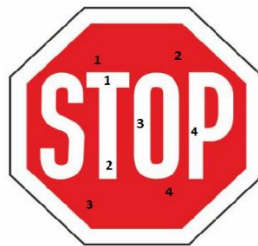
Figure 1: Retroreflection measurement points for STOP road sign.
