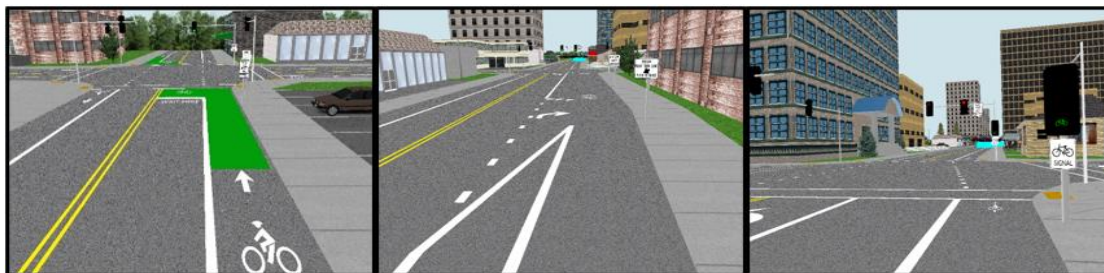
Figure 1: Bike Box, Mixing Zone, Bicycle Signal Treatments (from left to right)
