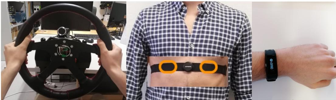
Figure 1 Placement of sensors: Cardiowheel (left), Movesense (center), PulseOn (right).
